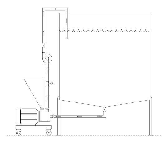
Example #2 describes the Inline SLIM System being used with a large (1000+ gallon) recirculation vessel. The Inline SLIM unit is located on ground level and is as close to the outlet of the tank as possible. Since the discharge tubing is long, a centrifugal pump is used to minimize the back pressure on the discharge side.
