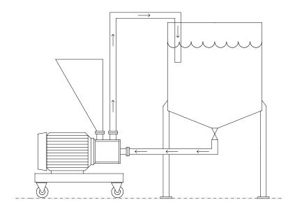
Example #1 describes the Inline SLIM System being used with a small (50 - 1000 gallon) recirculation vessel. The Inline SLIM unit is located on ground level and is as close to the outlet of the tank as possible. Discharge tubing length is kept to the minimum possible length.
